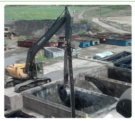
This mixing operation at the Yukon facility is covered under the existing hazardous waste permit. Here, wastes deemed hazardous are treated to adjust pH levels or chemically bind metals so that they don't leach. After treatment, the waste is analyzed to confirm it meets permit standards, and then is disposed of as residual waste.
