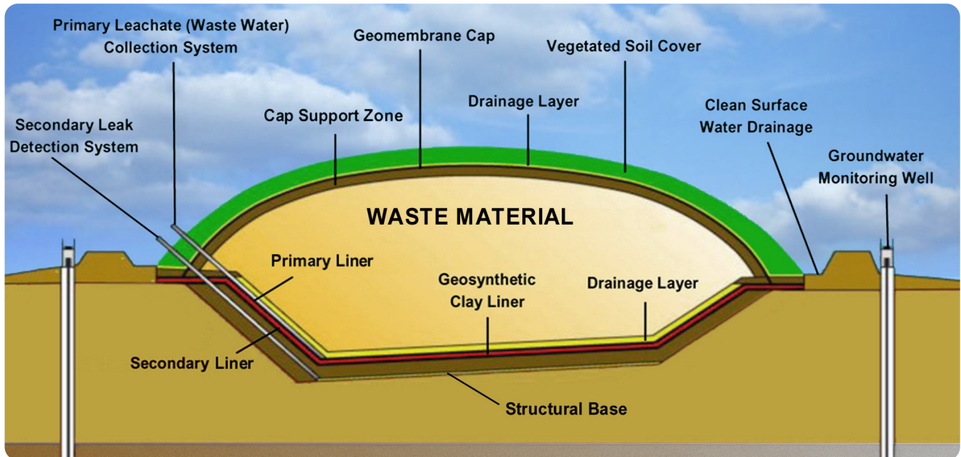
Typical cross-section of a Class 1 Residual Waste Landfill
