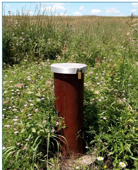
*Secured monitoring wells like this one are used to test the groundwater quality in and around the proposed landfill location.*
