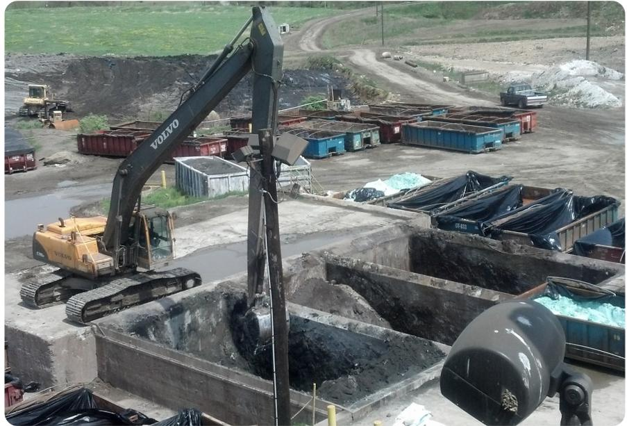
This mixing operation at the Yukon facility is covered under the existing hazardous waste permit. Here, wastes deemed hazardous are treated to adjust pH levels or chemically bind metals so that they don't leach. After treatment, the waste is analyzed to confirm it meets permit standards, and then is disposed of as residual waste.
