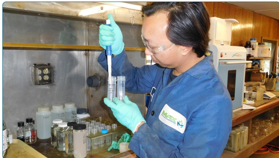
Jeffrey Funk, Ph.D., prepares waste samples for analysis to determine if the material meets landfill disposal criteria. Debris from the fire at Westmoreland Cleanways' Latrobe facility was similarly analyzed before being approved for disposal by DEP.
